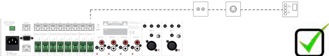
One Wall Microphone input (WMI) unit and one MWX65 Wall Panel can be connected on one Wall Panel Input. (The WMI audio input and MWX65 audio input are both using different pairs)
