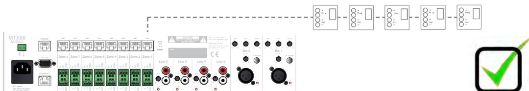
*Multiple MWX43/45 and one MWX65 Wall panel can be connected on one Wall Panel Input. They can be configured to control all the same, or different zones. The audio input of the MWX65 can only be routed to the zone its connected to.*
