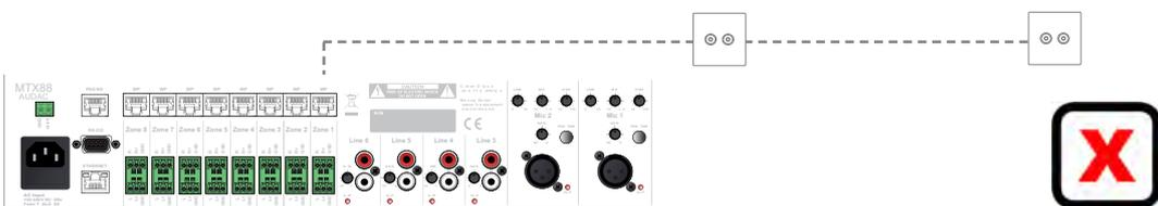
Multiple Wall Microphone input (WMI) units **cannot** be connected on one Wall Panel Input. (They use the same pair, both input 8)
