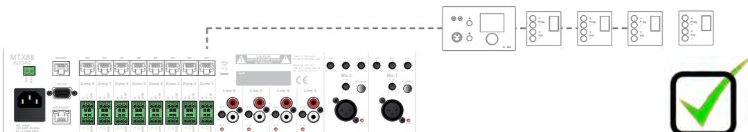
Multiple MWX65 Wall panel **cannot** be connected on one Wall Panel Input
