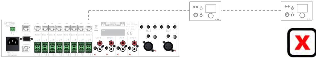
One Wall Line input (WLI) unit, one Wall Microphone input (WMI) unit and one (or multiple) MWX43/45 can be connected on one Wall Panel Input.
