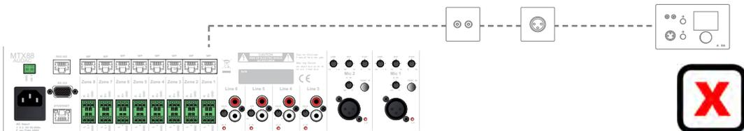
Multiple Wall Line input (WLI) units **cannot** be connected on one Wall Panel Input. (They use the same pair, both input 7)
