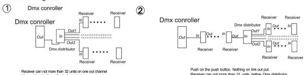
Receiver can not more than 32 units on one out channel
