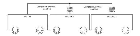
DMX input: from the DMX transmitting device DMX output: connect to the DMX receiving device
